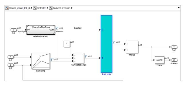
This link between the model and the generated code helps you identify the parts of your model that are causing defect. That way you can fix the defects in the model rather than the code.
