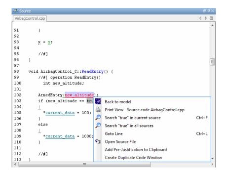
**Tip** For the **Back to model** command to work, you must have your Rhapsody model open.
